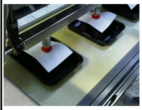
This machine automatically places pre-cut absorbent "Peach Pads" into pre-formed trays on a thermoforming system and can be easily changed between lane configurations. Spare magazines can also be supplied for different pad sizes. 2 and 3 row placing is an option.
