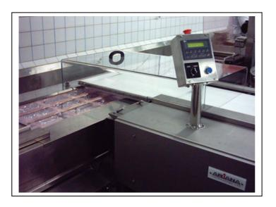
The **Jenton-Ariana** Multi Loader has been developed for the Red Meat Industry. A complete meat product handling system either incorporating the Jenton-Ariana Hi speed portioner for ground mince and diced meat loading or if fed from a slicing line, other meat products can be successfully packed. Can load semi rigid or flexible film for vacuum packs.
