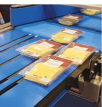
The Packleader BCS range of high speed convergers is designed to take multi-lane production of thermoformed packs and converge them at accurate spacing into a single lane.
